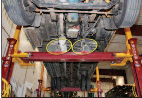
Chassis lifting beam permits vehicles to be raised by the frame, leaving the wheels hanging free.
