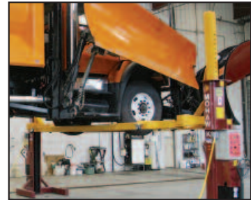
Wing plow adaptor permits snow trucks to be raised without the lengthy process of removing wing plows to gain access to the front tire for lifting.
