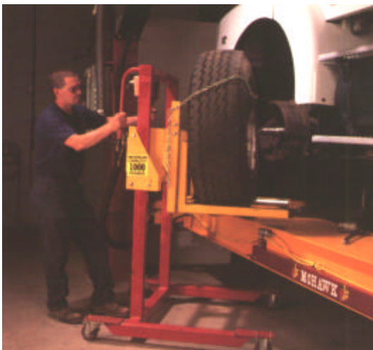
TD-1000 high rise tire dolly makes tire & brake work go faster even on the heaviest dual tires.
